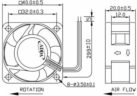
LEAD WIRES : UL 1007, AWG26, L = 295 + 10 mmRed = positive ; Black = negative.
