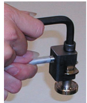
NMOHFTHKCRIMP For self-assembly, use the NMOHFTHKCRIMP tool to seal the solder joint cavity of the NMOHFTHK mount.
