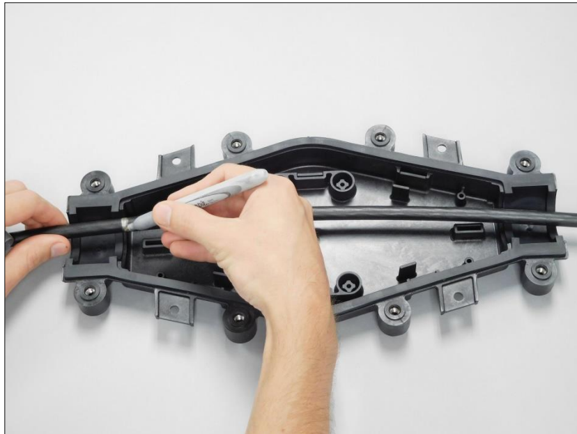
Figure 2-19. Cable marking in breakout box
