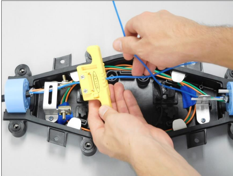
Figure 2-23. Using a mid-span entry tool to open appropriate buffer tube
